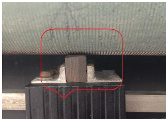
Figure 3: poor contacts in rheostats.
