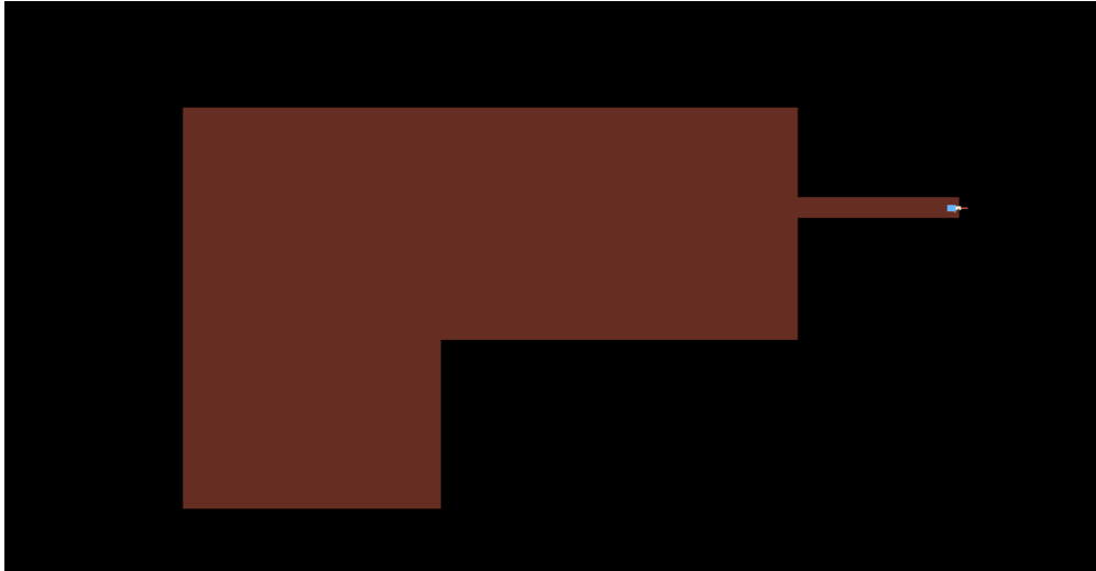
Figure1.5 Inverted L patch antenna
