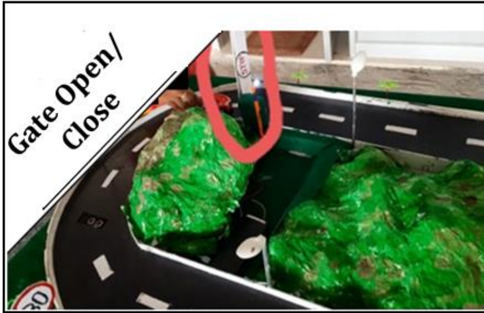
Figure 7: Gate open/close when vehicle reached at both end point
