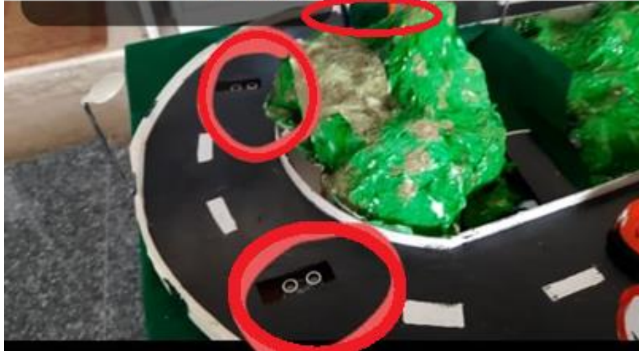
Figure 5: Sensor fixed to sense the vehicle and vehicle speed
